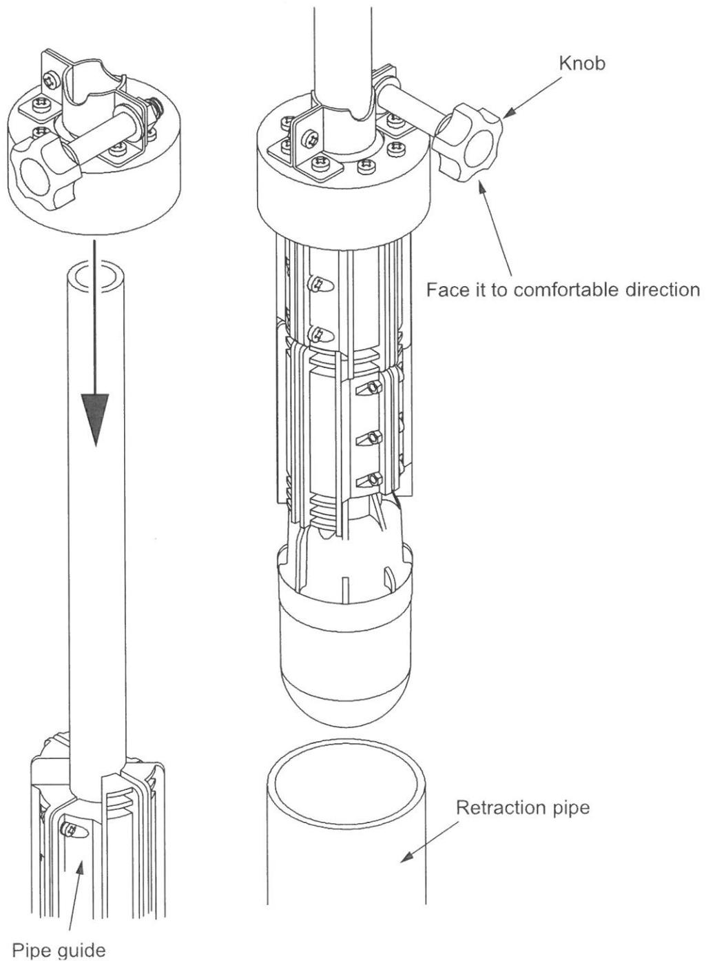
9. Lower the storage pipe cover until it hits the tank guide followed by tightening the knob.
