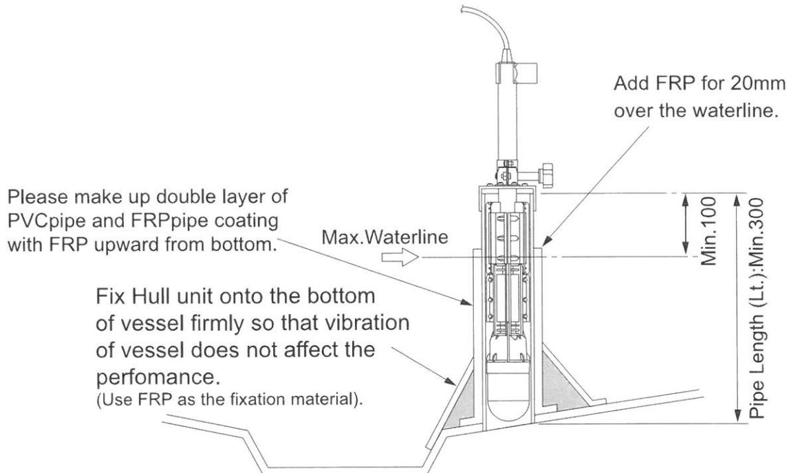
Add an extruding part of approx. 5mm with FRP for the purpose of reducing the water pressure inside the pipe while sailing.
