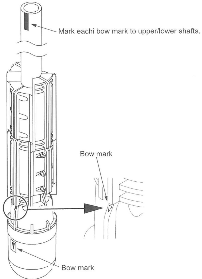
8. Loosen the knob of storage pipe cover so that the shaft goes through it.
