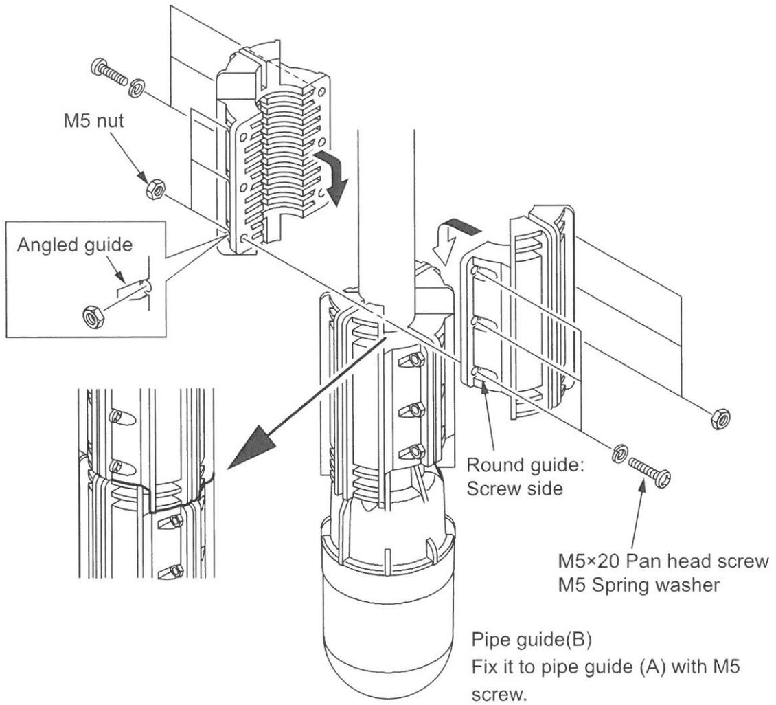
※No need to use pipe(tank) guide (B) if pipe length is less than 410mm.
