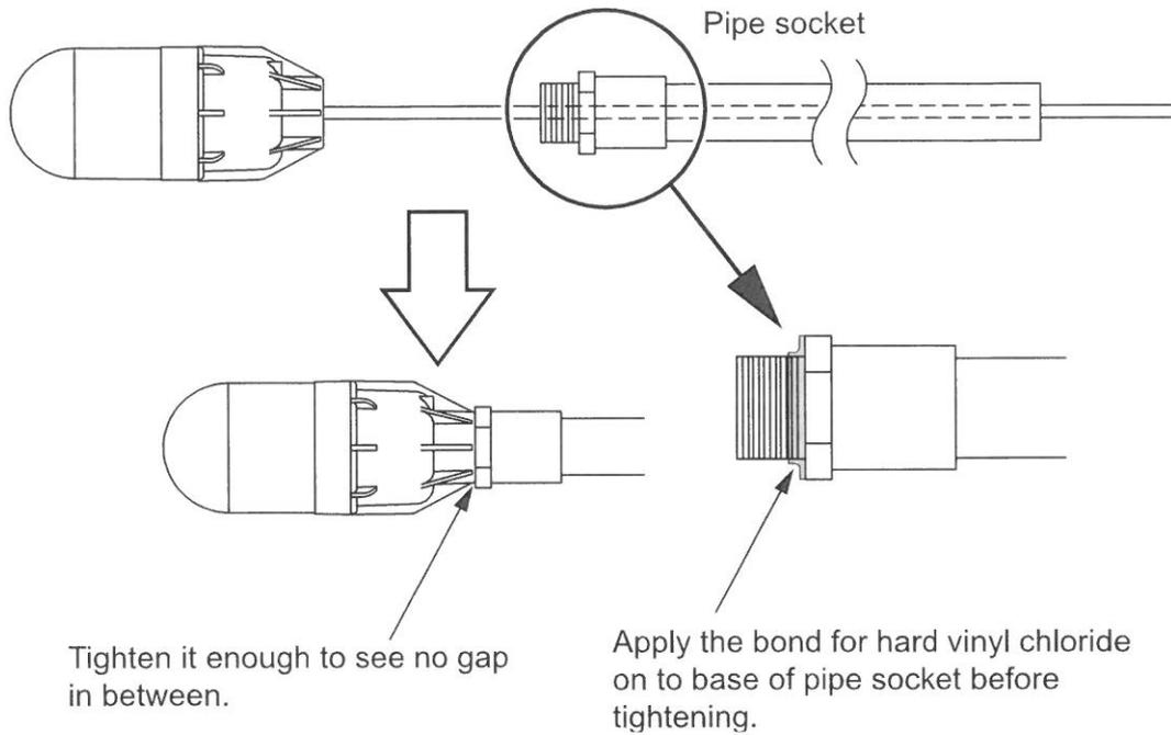
5. Fix Upper/Lower shaft and transducer with pipe(tank) guide(A).
