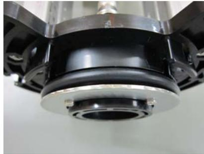
Insert the rubber bush into transducer part.
