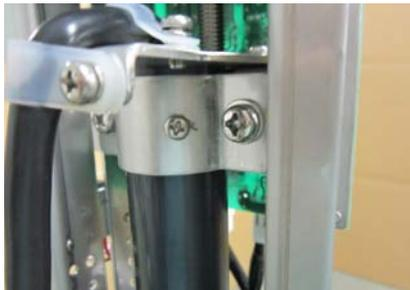
Remove the cable clamp and fix the cable.
