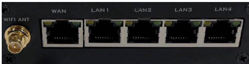
Figure 5.4.b - Wi-Fi antenna connector / WAN Port / LAN Ports 1, 2, 3, 4
